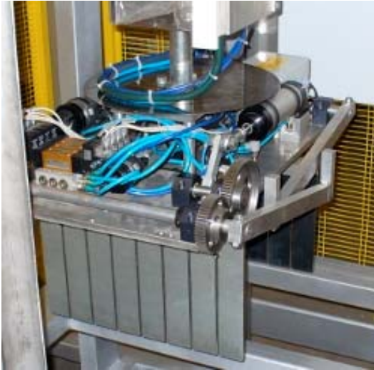
Self-centering gripper 400 with pallet hooks
