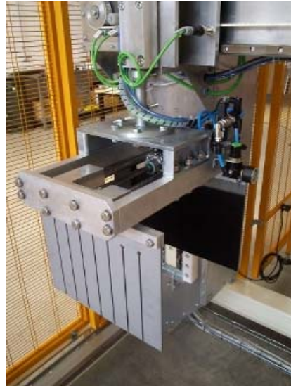
Gripper with a fixed and a movable flap
