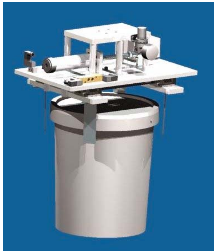
Self-centering gripper with hooks for buckets
