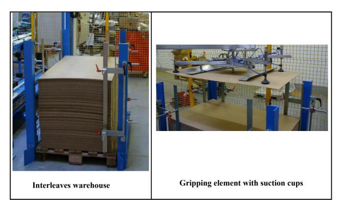
The column pallet interleaf feeder consists of a vertical column, two arms and a gripping head of the interleaf. The pallet interleaf feeder engages the brim with 4 suction cups, the user raises a fixed amount and the door into position above the pallet. The flap is positioned over the pallet construction.
