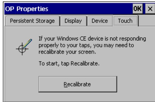
Recalibrate the Windows CE unit screen if your input is not correctly executed.
