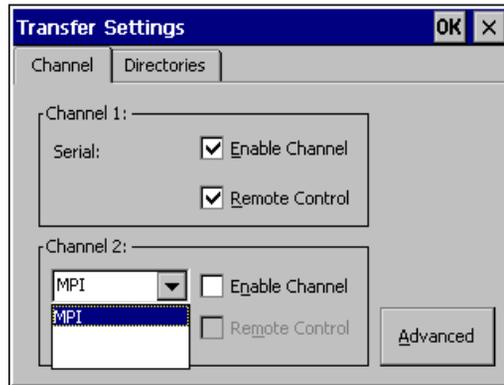
Figure 3-4 Transfer settings configuration menu, *Channel* tab control, TP 170B and OP 170B
