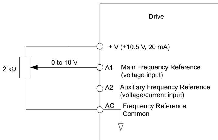
**Figure 5.1 Setting the Frequency Reference by Voltage Input**
