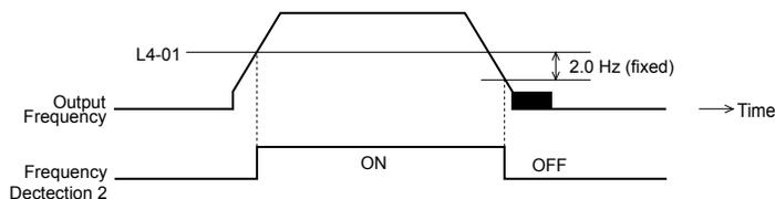
Figure 5.84 Frequency Detection 2
