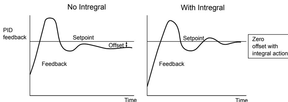
Figure 5.19 Offset Elimination by Integral Operation
