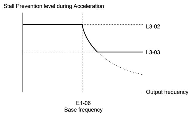
Figure 5.81 Stall Prevention Level and Limit During Acceleration
