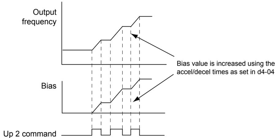
Figure 5.37 Up/Down 2 Bias when d4-03 = 0.0 Hz
