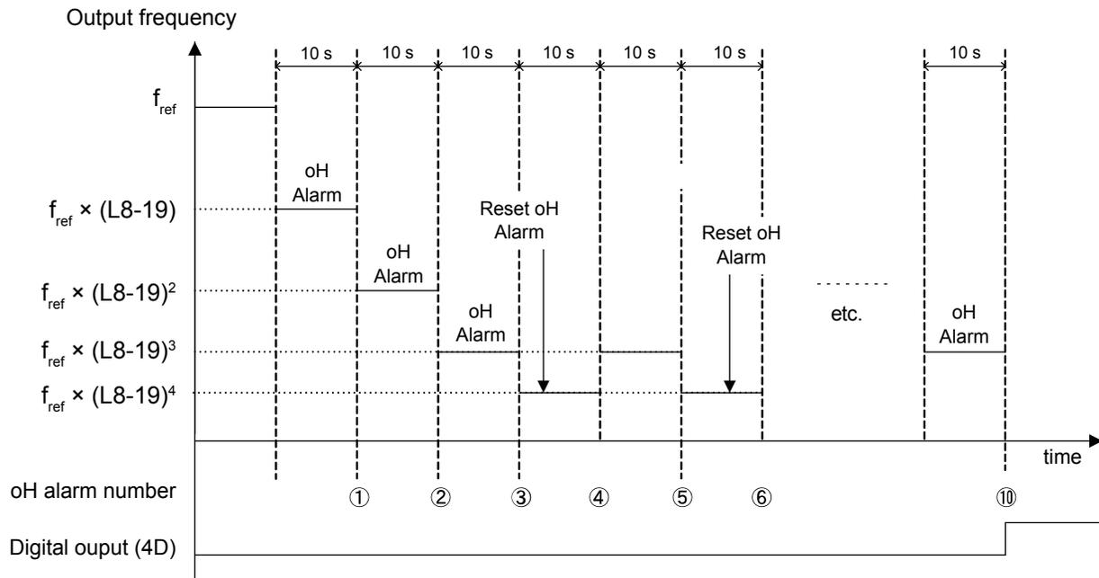
Figure 5.88 Output Frequency Reduction During Overheat Alarm
