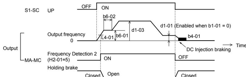
Figure 5.85 Holding Brake Time Chart
