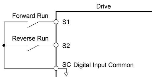
Figure 5.51 Example Wiring Diagram for 2-Wire Sequence
