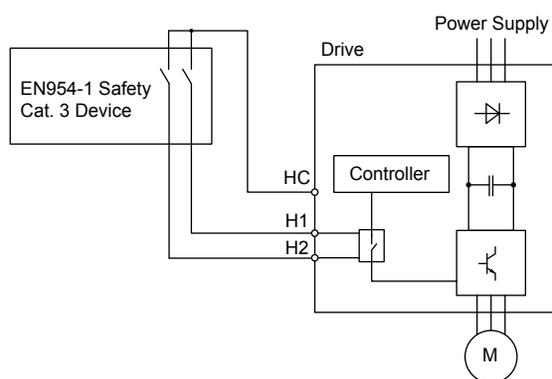
Figure D.9 Safe Disable Wiring Example
