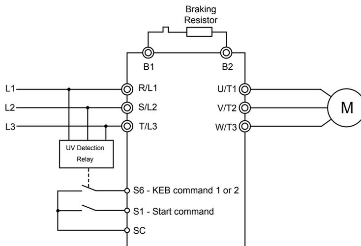
**Figure 5.78 KEB Function Wiring Example**
