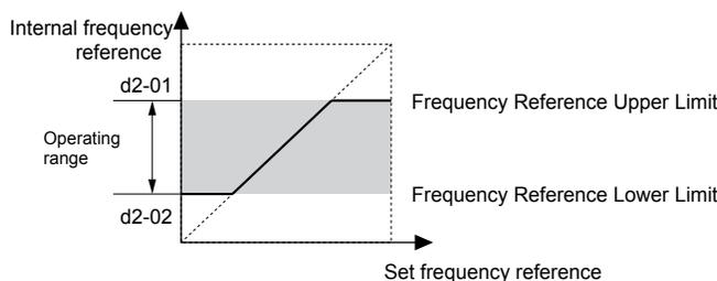
Figure 5.32 Frequency Reference: Upper and Lower Limits
