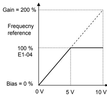
Figure 5.68 Frequency Reference Setting by Analog Input with Increased Gain
