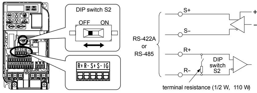
Figure C.5 Serial Communications Terminal and DIP Switch S2
