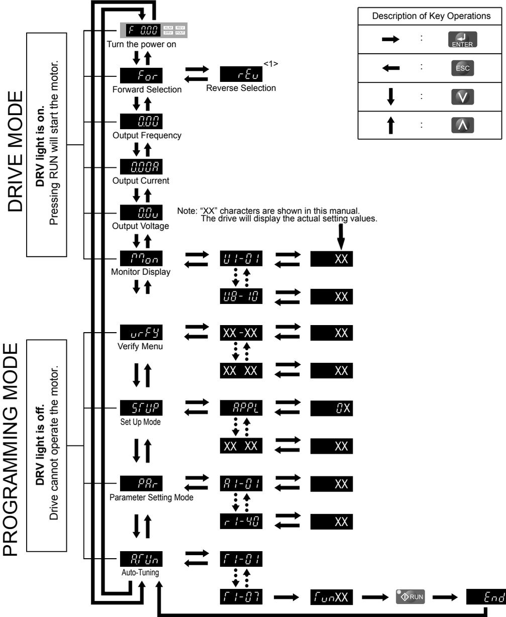
Figure 4.3 Digital LED Operator Screen Structure
