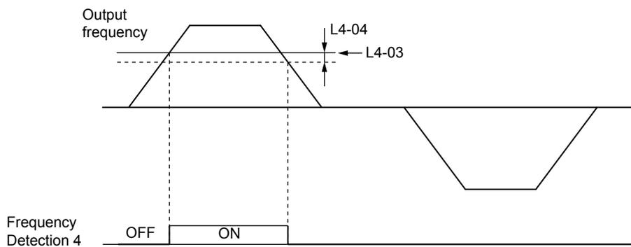
Figure 5.62 Frequency Detection 4 Example with Positive L3-04 Value
