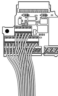
Figure 7.8 Removable Terminal Board disconnected from the drive
