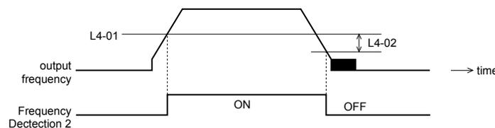
Figure 4.10 Frequency Detection 2
