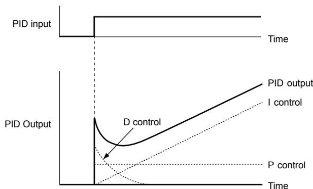
Figure 5.17 PID Operation
