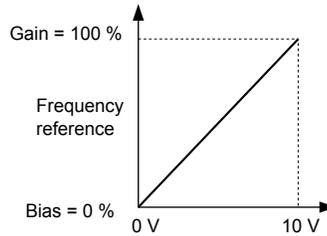
Figure 5.67 Analog Input A1 Default Characteristics
