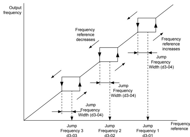
Figure 5.33 Jump Frequency Operation
