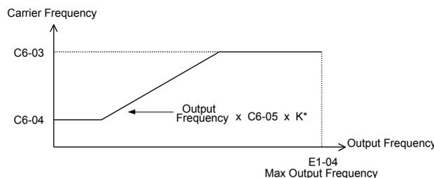
Figure 5.29 Carrier Frequency Changes Relative to Output Frequency
