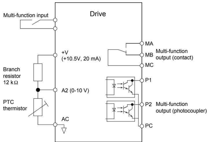
Figure 5.75 Connection of a Motor PTC
