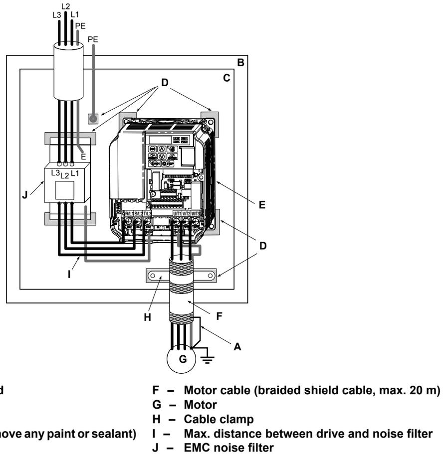
Figure D.4 EMC Filter and Drive Installation for CE Compliance
