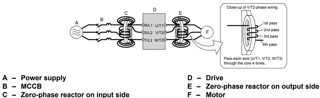
Figure 8.10 Zero-Phase Reactor
